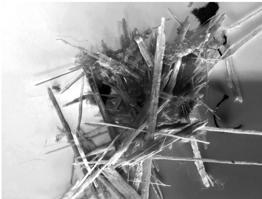
Fig. 1. Complex and inhomogeneous material from the shredded wind turbine blade
